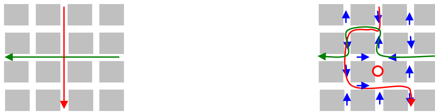
Figure 15: Scheme of non-regulated traffic and traffic operating in a system of restricted roads
